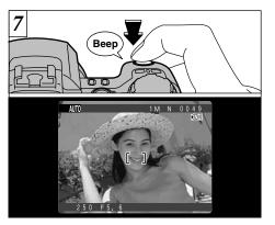
If you press the shutter button down halfway and then press the shutter button down fully without releasing it, the camera beeps once and takes the picture. The "" icon then appears on the screen and the shot is recorded as an image file.
